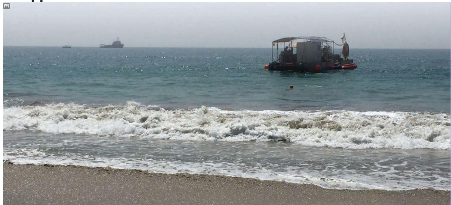
MB3 is a self-propelled modular shallow water multipurpose Pontoon specially constructed to support the SKORPIOS Series Jet Trenchers and the related diving operations. It can be transported in sections on one 40ft standard size trailer, and assembled into a working platform in three hours and be fitted with various configurations of installation equipment. The barge is expandable to easily accommodate larger loads.
