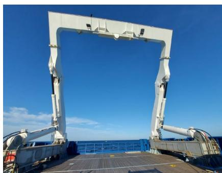
**The 35-ton A-Frame** has the following dimensions: 7.5 m of maximum outreach (from the vessel), 13.95 m width x 11.95 m height. **The AHC crane with 25T@8m** allows for construction support works: mattresses and rock bags installation, etc.
